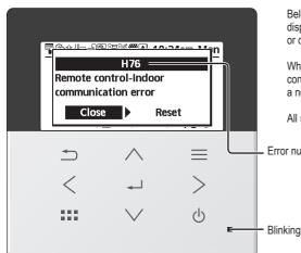
Below is a list of error codes that may appear on the display when there is some trouble with the system setting or operation.
