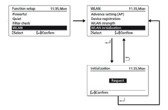
When Initialization finish, WLAN LED will off automatically.
