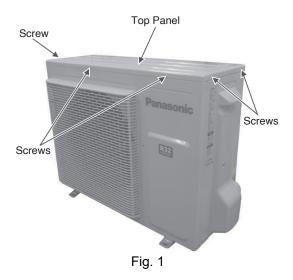
2 Remove the 8 screws of the Front Panel.
