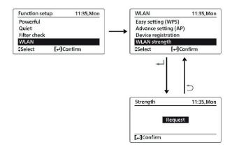
• After 5 seconds, the signal strength is shown on the indoor unit WLAN LED.
