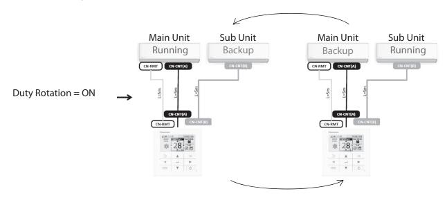
2. After rotation interval ends, Main unit will be turned off (becomes backup unit) and Sub unit will be turned on (becomes running unit) for the next rotation cycle. Role of running and backup unit will rotate between Main and Sub unit for each new rotation cycle.
