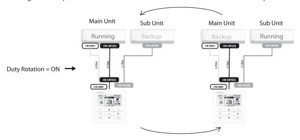
Figure 1.2 Rotation of running/backup unit roles between Main and Sub unit
