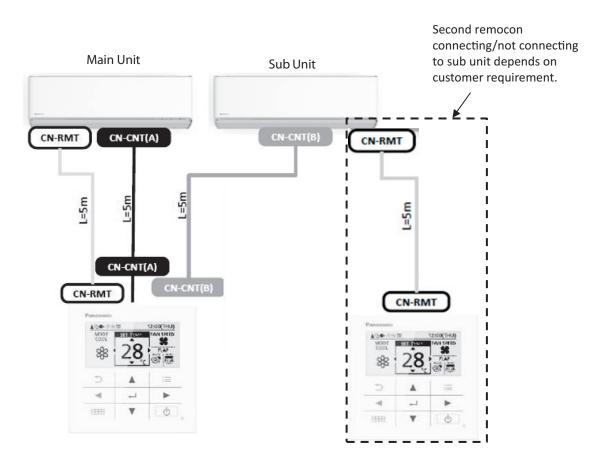
Figure 1.1 Duty rotation system outline showing Main unit, Sub unit, CN-RMT and CN-CNT
