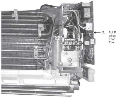
Pull PCB half way then remove all connectors, CN-WHT from PCB. Then Remove main electronic controller. Then remove PCB.
