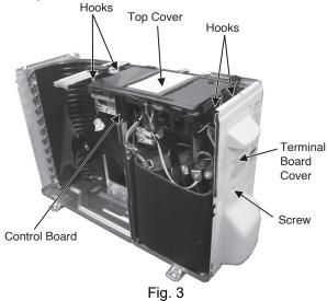
5 Remove the Control Board as follows:
