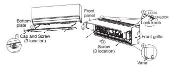
Upper vane: Set to horizontal: Lower vane: Set to slightly below horizontal Model Z50\*\*\*, Z71\*\*\*
