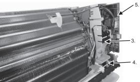
Pull out the Main Electronic Controller halfway. Then disconnect all connectors from the controller. Remove the Electronic controller.
