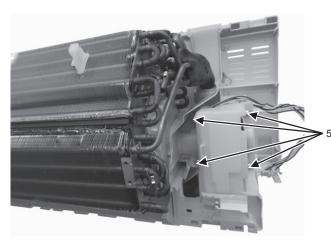
Remove 4 screws from fan motor cover.
