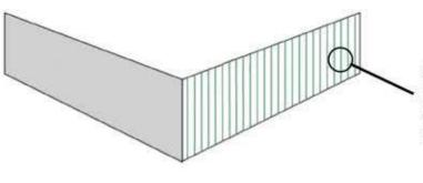
Spread plaster with a toothed spatula from top to bottom. We recommend using a spatula with tooth gaps of 10 mm. Any possible moisture will flow down the tracks.
