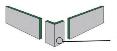
First install the corner piece. Then continue installation with full-sized panels.
