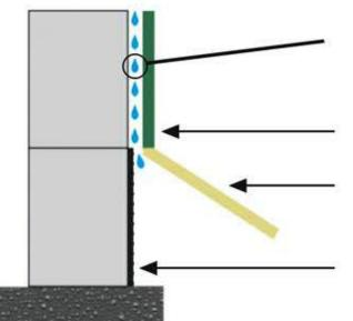
Any moisture that forms behind the panel will flow down the tracks in the plaster.
