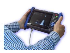
IP camera tester is great CCTV tools for IP camera's installation and maintenance, both for Analog and IP camera test, built in video level meter, Analog and digital video signal output, IP address scan, Ping test, Port flashing, cable test, Digital Multi-meter, optical power meter and TDR cable tester etc, very easy to operate
