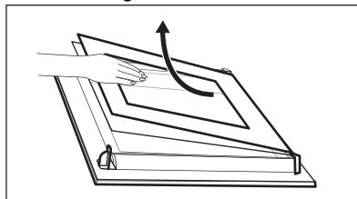
4. Clean the door glass panels. To install panels, do the same steps in reverse.
