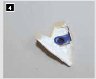
4 The centre spike serves as centering for the 68 mm diameter drill bit.
