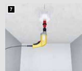
The individual hole is drilled with a hole cutter...
