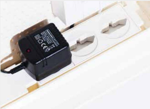
The hardware components are fixed to the plastic equipment racks, potential-free, and supplied from the mains via the triple socket.
