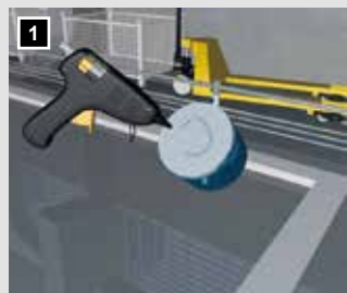
Glue XL 170 large box with hot glue on the sound table.
