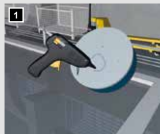
Glue 306 mm diameter lower part/co- ver with hot glue onto the sound table.
