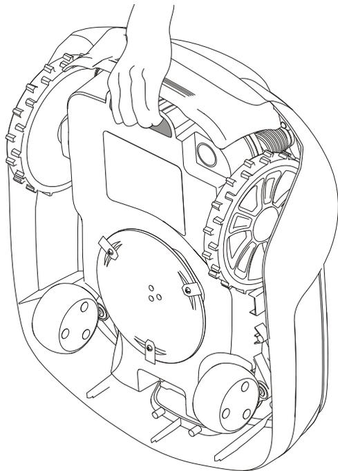
Press the **STOP** button and remove the safety key before lifting.
