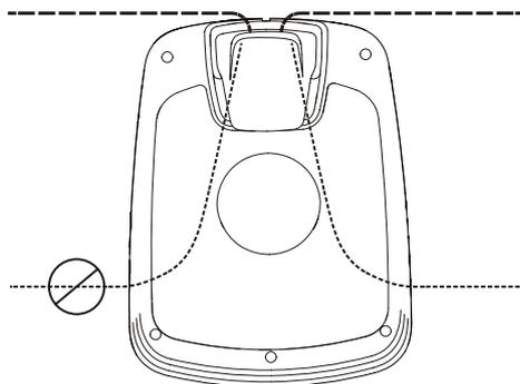
The entire charging station must be inside the operating area as shown in the figure.
