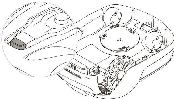
Press the **STOP** button on the mower and remove the safety key.
