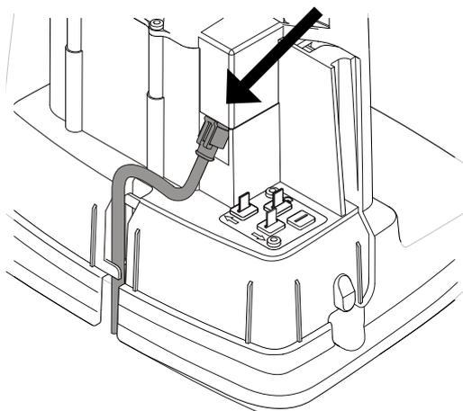
Connect the low voltage cable to the charging station.
