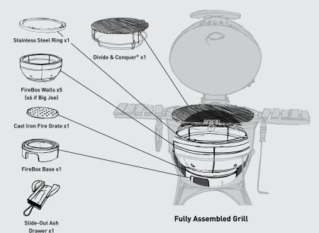
4 Begin building the FireBox Walls. Place each piece on top of the FireBox Base. Note: the pieces will lean against the inner wall of the base of the grill.
