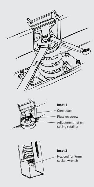
TOOLS REQUIRED: 10MM OPEN END WRENCH OR 7MM (OR 9/32 INCH) SOCKET WRENCH, DEPENDING ON THE MODEL. 19MM OPEN END WRENCH (OR 3/4 INCH OPEN END WRENCH)
