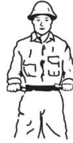
4. PULL THE TIP OF THE BOOM IN Both fists in front of your body, thumbs pointing inward.
