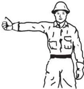
1. RAISE THE BOOM TIP Arm extended, fingers closed, thumb up.
