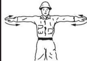
8. EMERGENCY STOP With both arms extended, palms facing down, move your arms back and forth horizontally.
