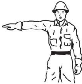
5. SWING With your arm extended, point your finger in the direction of the boom swing.
