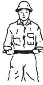
3. STRAIGHTEN THE BOOM TIP Both fists in front of your body, thumbs pointing outwards.
