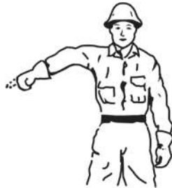
6. USE THE GRIP With your arm bent and fingers pointing downwards, open and close your fist.
