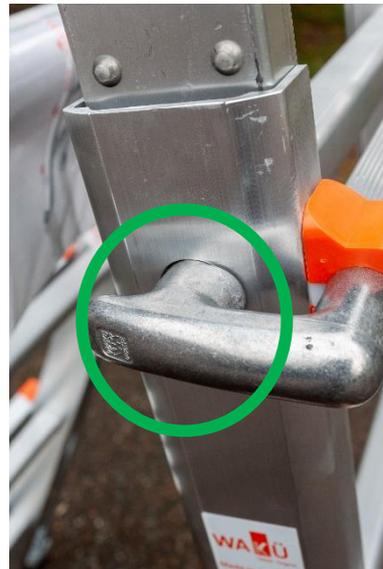
Height adjustment handle is correctly locked.
