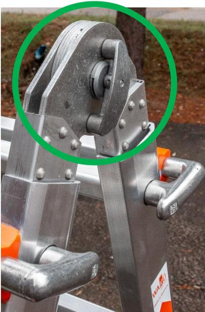
Lock the pins again before you climb the ladder. The lock should make a clicking sound.
