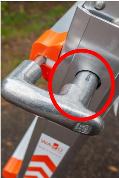
Height adjustment handle is not properly locked.
