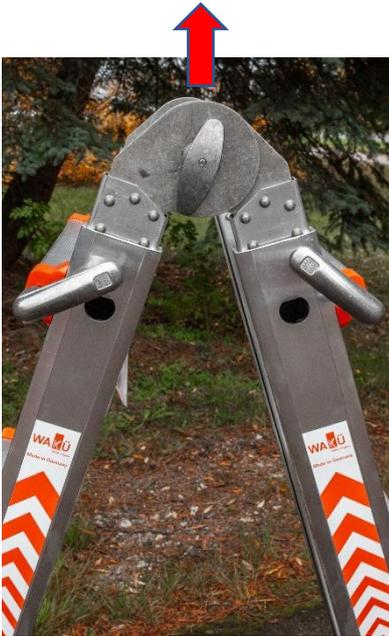
Pull the adjustment handles out on both sides (see picture). Raise or lower the inner part to the desired height and push the handles back in, making sure that they lock correctly. Locking is possible at each rung, as there are holes that allow the handle to be pushed into the inner ladder.
