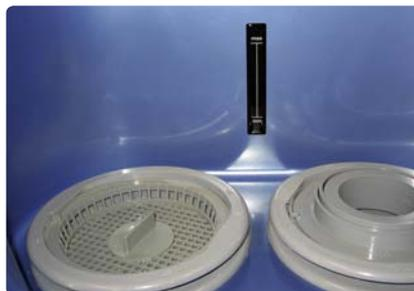
**After draining, always fill the minipool through the filter canister. Otherwise air may remain in the pump and hinder it from creating a water circulation. Water level should cover filters at least by 10 cm.**
